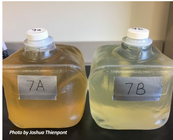
Fig. 3 Water samples from two nearby, paired lakes showing differences in water colour / DOC with thaw slump presence. The lake with no slump (7A) is highly stained, while the lake with a slump (7B) is relatively clear.
